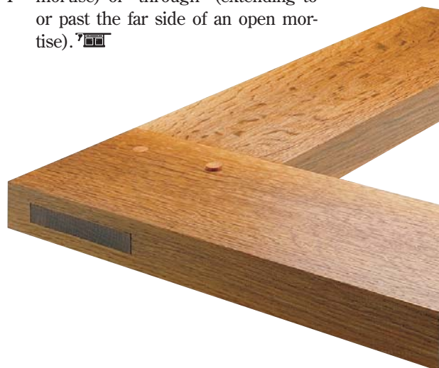
6 Use a clamp to close the joint, then check the assembly for square. Drive the pegs with a deadblow or wooden mallet.
